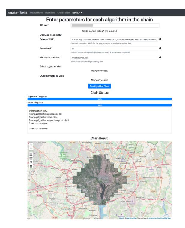
When the chain runs, you'll see some status information and a progress bar indicating how far along the chain we are. An algorithm developer can also pass algorithm progress to the user as we'll see in another section.
