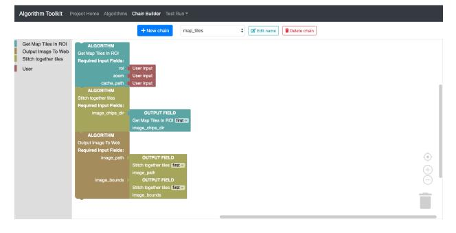
The left side of this screen contains the algorithms installed in your project. To the right of that and taking up most of the screen, is the Chain Builder Canvas. As you can see, "map\_tiles" links the algorithms together in the following order (top to bottom):
